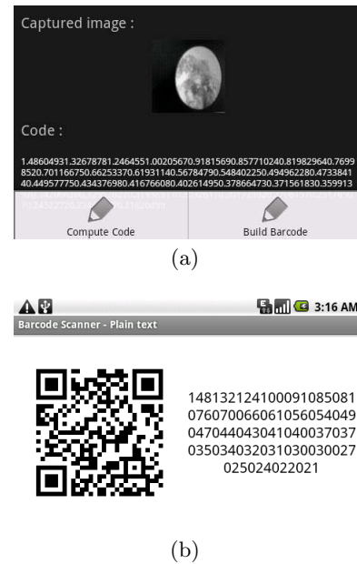
Figure 9: (a) A speckle image taken on the cellphone and the fingerprint of the speckle image; menu options: i) Compute Code, or ii) Build Barcode. (b) QR code of the fingerprint which is shown on the right side.
